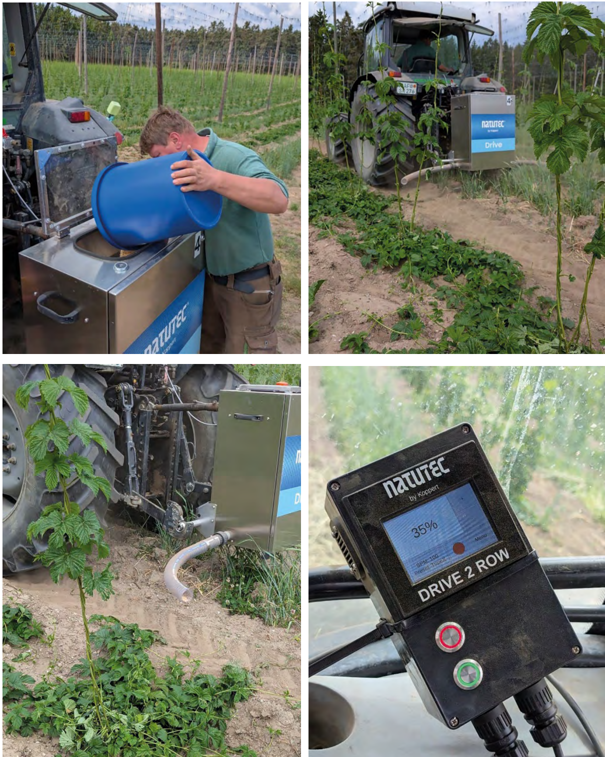
Figure 2. Details of the technical release method for predatory mites in hops. Above, left: Infilling of the mite mix with sawdust as a carrier in the Natutec Drive funnel; right: application in the field; below, left: detail of application; right: control unit for the Natutec Drive device in the operator's cab; Eichelberg, 21.v.2025. Photos: FW
